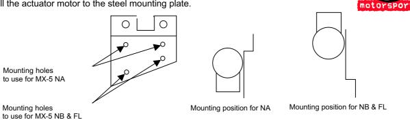
Unscrew the fixing nuts for the trunk key lock and mount the steel mounting plate and motor here.
